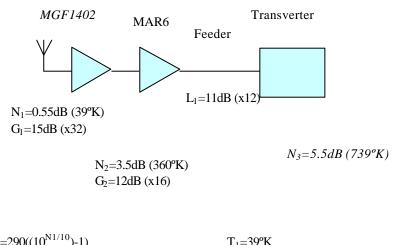
$\begin{array}{l} T_1 = 290((10^{N1/10}) - 1) \\ T_2 = 290((10^{N2/10}) - 1) \\ T_3 = 290((10^{(L1+N2)/10}) - 1) \\ T = T_1 + T_2/G_1 + T_3/(G_1G_2) \end{array}$
